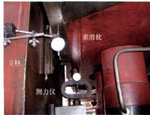
图4 静态测力试验现场 Fig.4 Static experiment site of force measuring
